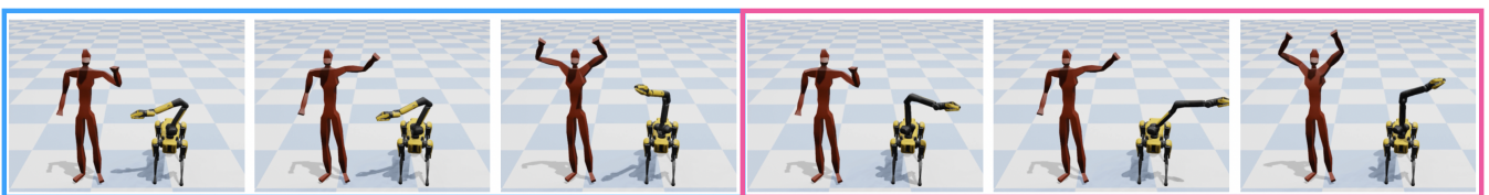
Fig. 5. Different generated Spot Wave motions by varying end-effector mapping. The blue uses auto-mapping while the pink one is manually assigning Spot's manipulator with human left arm.
